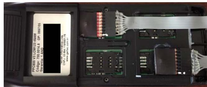
Fig. 5. The compartment at the bottom of the PPC800 PIN-pad, with the two accelerometers glued over two SAM (Security Authentication Module) slots.
