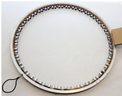
Fig. 1. Prototype of the “hula hoop” scanner. We mounted 36 ultra-sound distance measuring sensors at the inner side of a bicycle rim. At right, there is a board with auxiliary circuitry and connectors to the Arduino.
